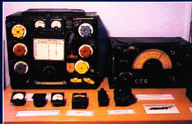
T1154 & R1155 were the transmitter and receiver used in most heavy aircraft such as the Lancaster
