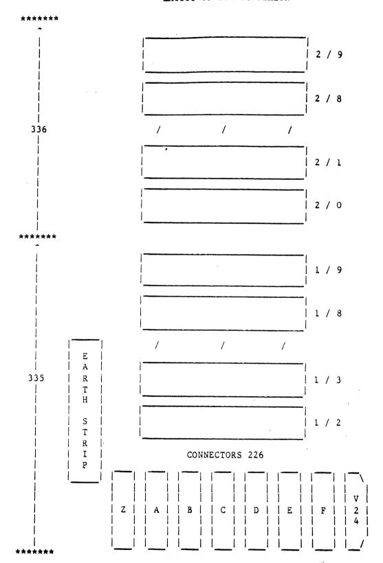
Connector Z is provided to cater for slots 1/2 and 1/3 plus V24 interface.
