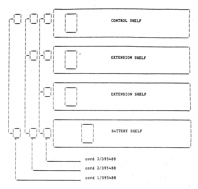
The above diagram shows the interconnexion of the 50v battery supply leads and the necessary connexion cords for a one, two or three shelf system.
