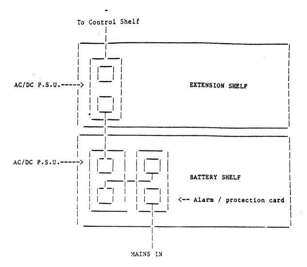
The above diagrams show the mains cable assemblies required for different system configurations. N.B. the mains cable always enters at the battery shelf and is connected directly into the Alarm / Protection card. It is then fed from this card into its AC/DC P.S.U.(if fitted) and then into the power supply unit of the next shelf above.
