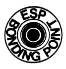
**Note** The connectors used are to a BT standard for ESP use only. The male connector will be fitted as an ESP bonding point on all new static sensitive BT equipment.
