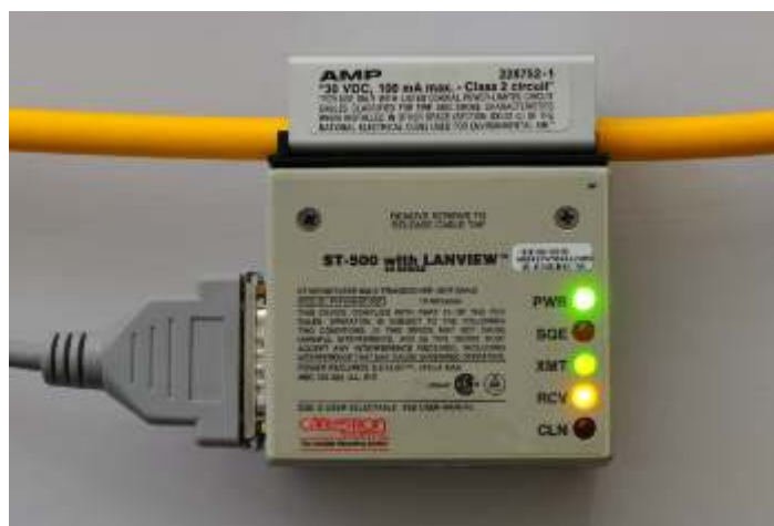
Fig. 8 Cabletron ST-500's (90 Series) MAU [mattmillman.com]
