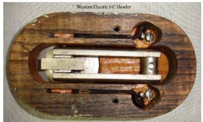
Western Electric's Howler No 1-c. The larger of the two offerings. Right: Rear view showing that this model is based on a Bell receiver with the magnet folded over within the wooden mounting block.
