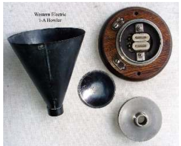
Western Electric's Howler No 1A. The smaller of the two offerings
