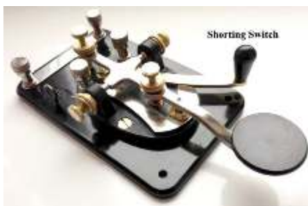
Morse key showing the shorting switch (top right)
