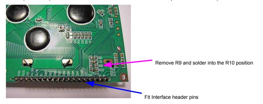
You will need to use a magnifying glass and tweezers to move the resistor. (if you cant successfully place it in the R10 position, just use a solder blob to bridge the two solder pads for R10 instead).
