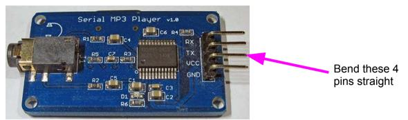
Bend the 4 header pins straight ready for attachment to the main board.
