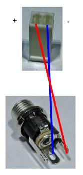
Use heat-shrink tubing over the entire socket to cover the connections after soldering.
