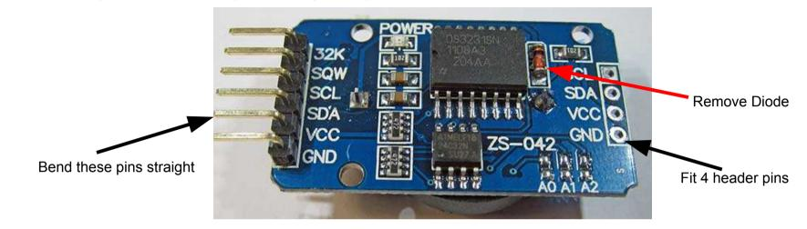
The glass diode (shown) must be **removed** as the module manufacturer originally provided it to charge a supercapacitor instead of the lithium coin-cell currently being used.
