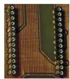
9. Solder the "D-Sun" voltage regulator to the board with its component side facing down and the white arrow pointing towards the diode D6
