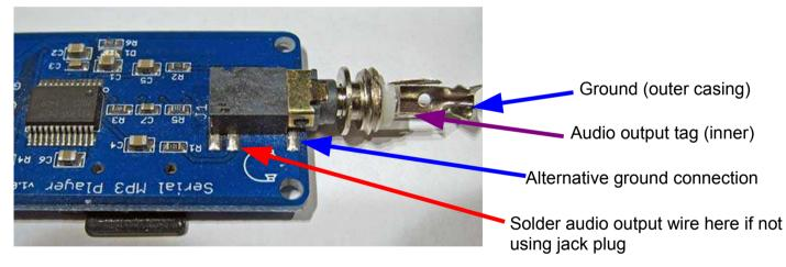
Plug a 3.5mm stereo jack plug into module (without the outer plastic cover) The output can later be wired via the centre jack plug tag or alternatively the jack plug can be omitted and the output wire soldered to the PCB pad as shown.
