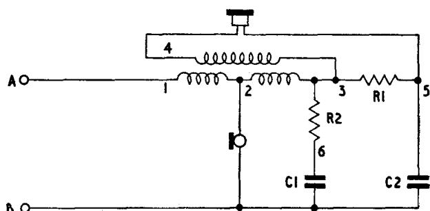
Fig. 8.-Circuit of "G.E.C. 1000" Telephone drawn in hybrid form.
