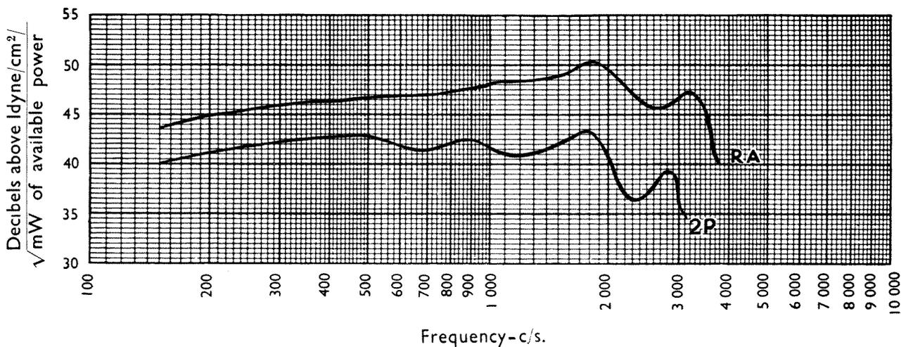
*Fig. 4.-Receiver frequency response.*
