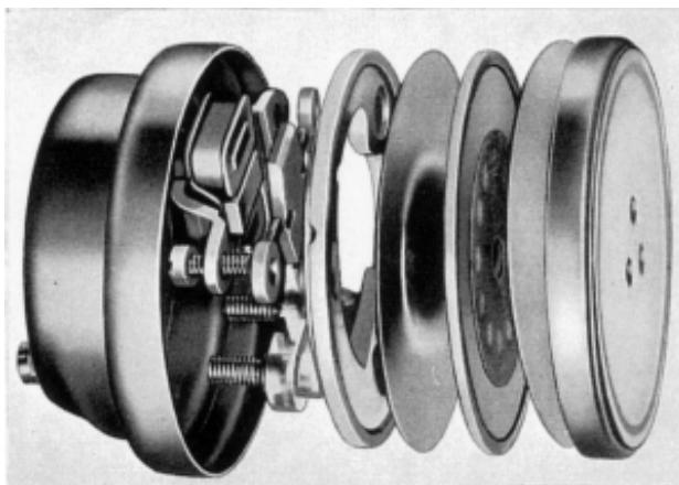
*Fig. 5.-Exploded view of rocking-armature receiver.*
