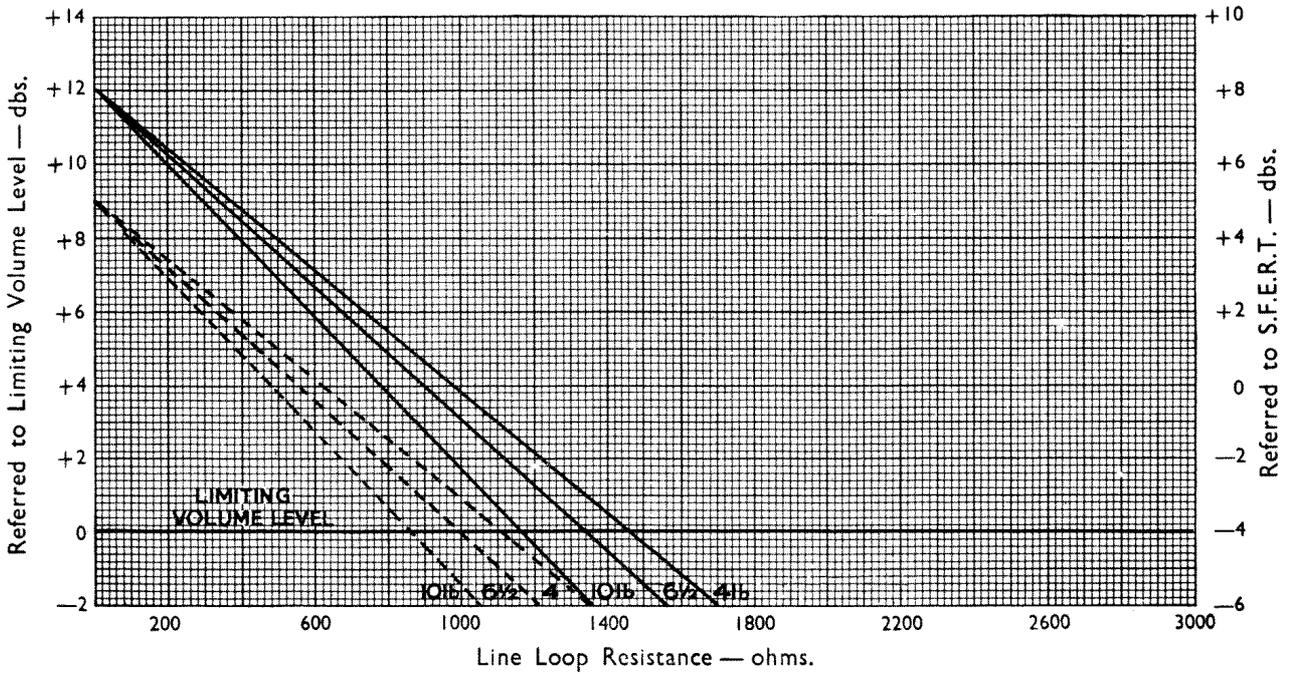
*Fig. 11.-Volume ratings for the telephone-receiving.*
