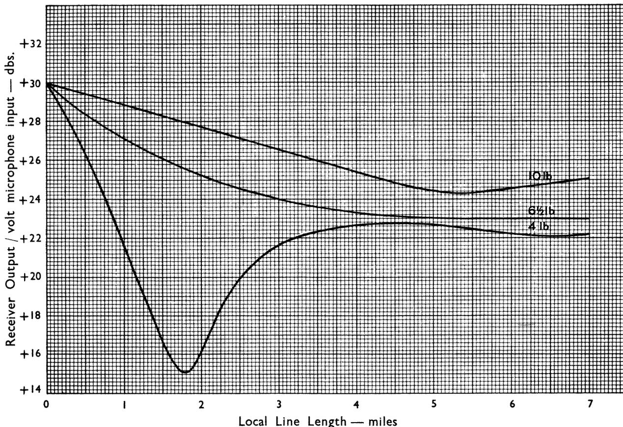
*Fig. 14.-Sidetone levels for the telephone.*
