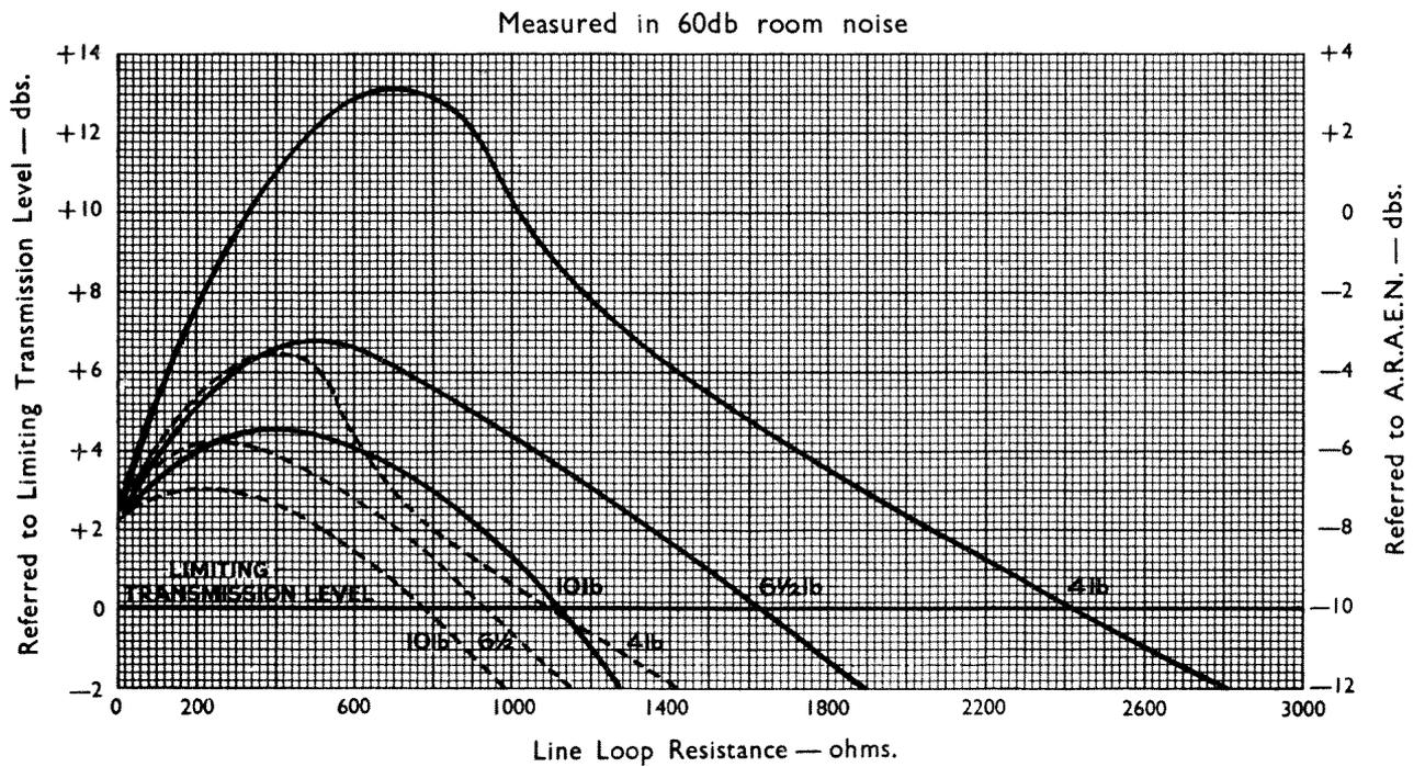
Fig. 13.-Articulation ratings for the telephone-receiving.
