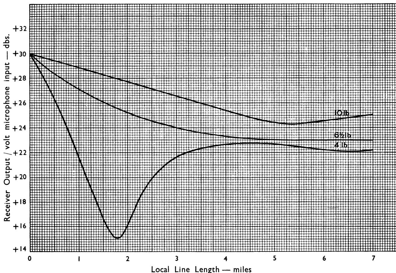
*Fig. 14.-Sidelone levels for the telephone.*
