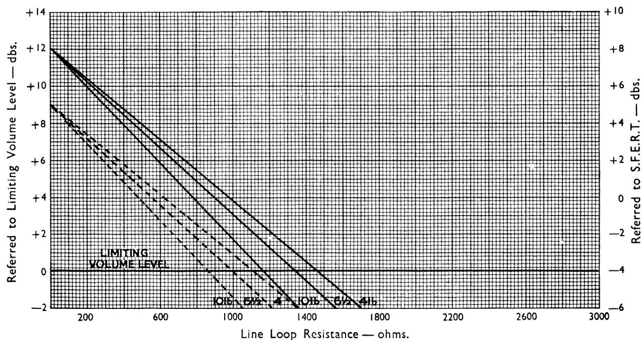
Fig. 11.-Volume ratings for the telephone-receiving.
