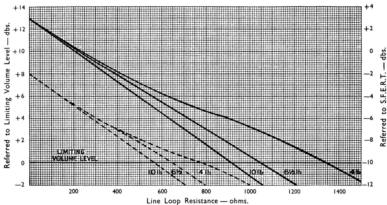
Fig. 10.-Volume ratings for the telephone-sending.
