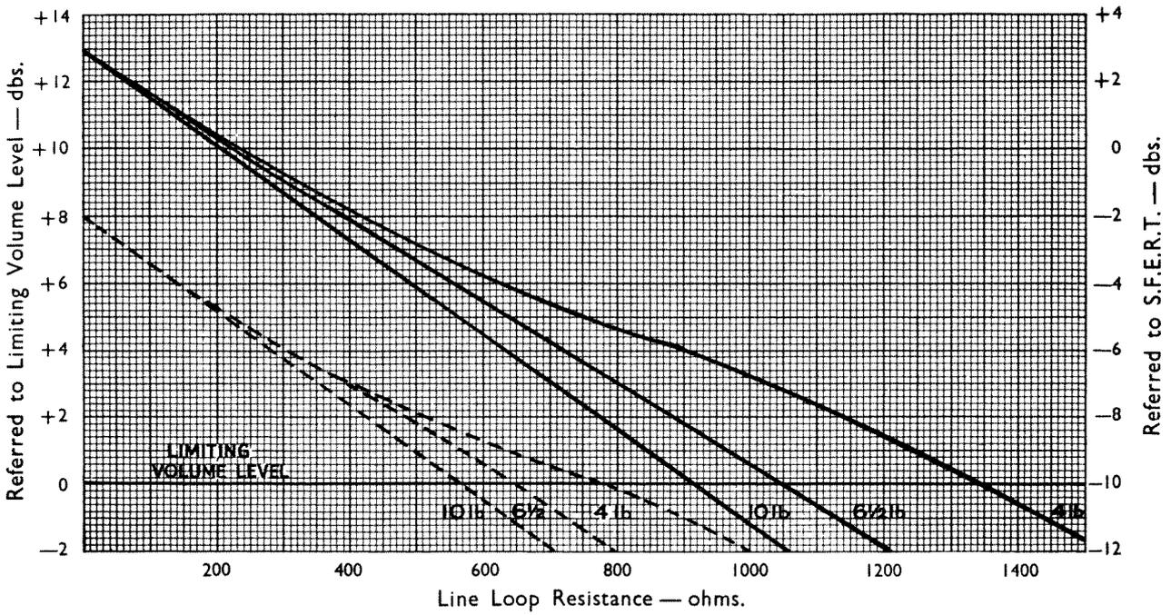
*Fig. 10.-Volume ratings for the telephone-sending.*
