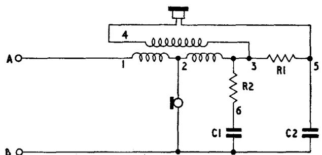
*Fig. 8.-Circuit of "G.E.C. 1000" Telephone drawn in hybrid form.*
