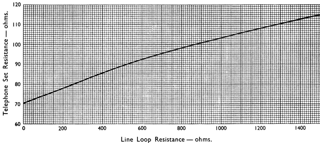
*Fig. 9-Variation of talking resistance with length of line.*
