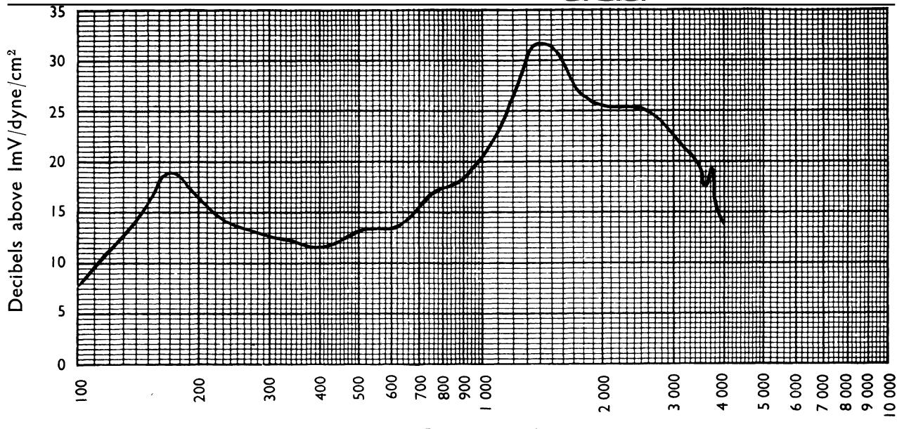
*Fig. 3.-Transmitter frequency response.*
