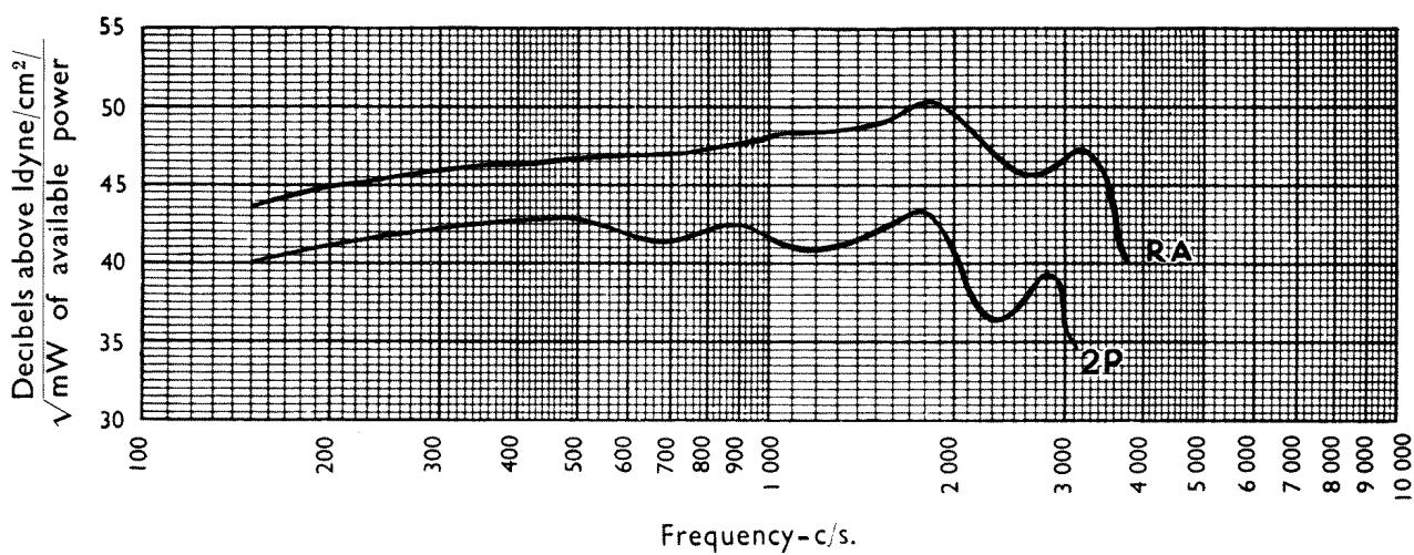
*Fig. 4.-Receiver frequency response.*
