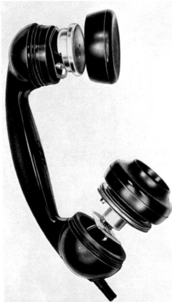
can be reduced by restricting granule agitation in the direction of current flow, but increased restriction results in decreased output from the transmitter. The inset establishes an appropriate balance and thereby gives a very high output consistent with an acceptable frequency response; together with a satisfactory signalling resistance.
