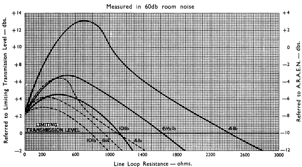
Fig. 13.-Articulation ratings for the telephone-receiving.
