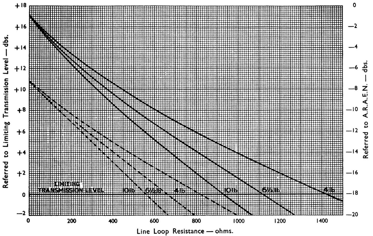
Fig. 12.-Articulation ratings for the telephone-sending.
