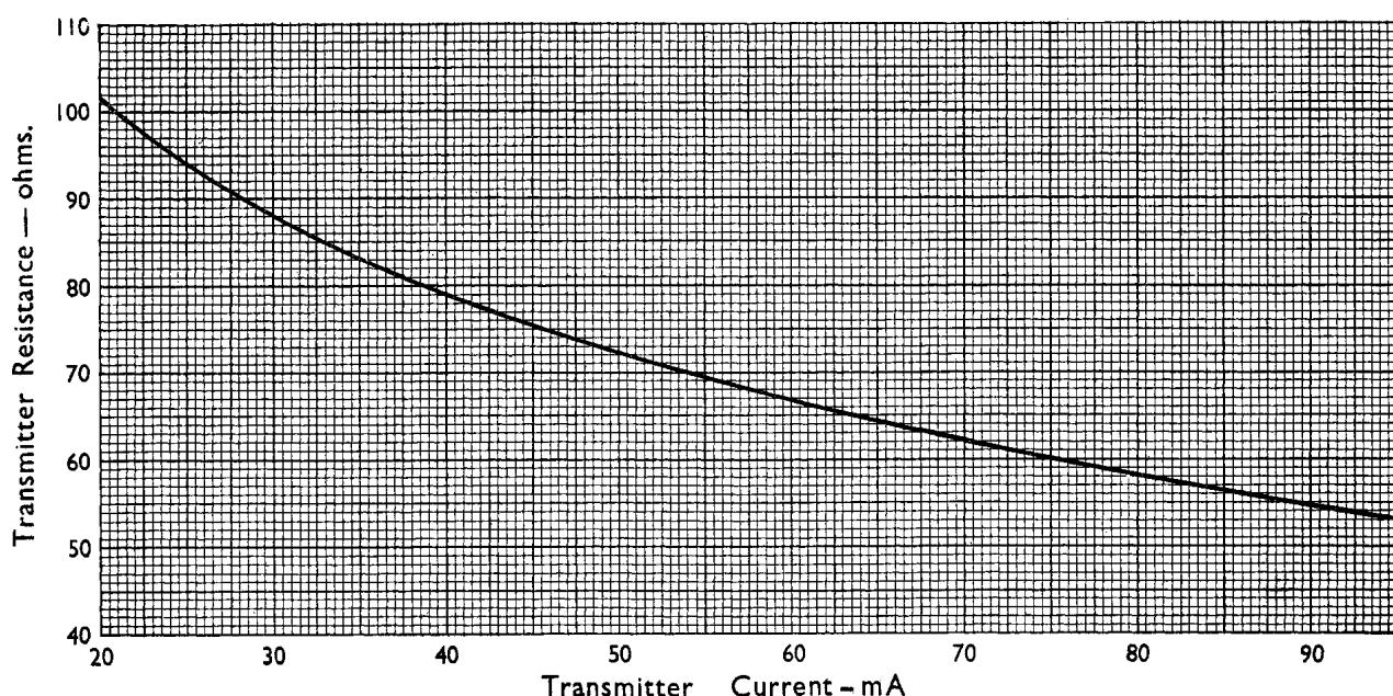
*Fig. 2.-Variation of transmitter resistance with current flowing.*
