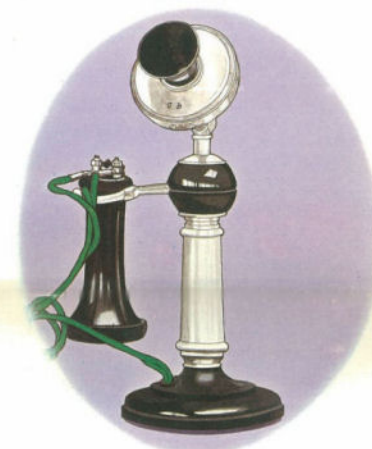
Called 'candlestick' telephones because of their shape, these were used from the 1880's for over half a century. Later models had dials. 1905
