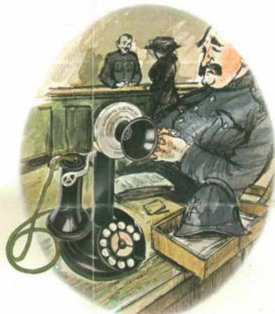
Called 'candlestick' telephones because of their shape, these were used from the 1880's for over half a century. Later models had dials. 1905
