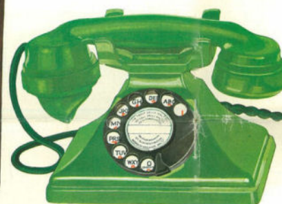
Plastic telephone with improved transmitter that solved the handset problem. 1929.
