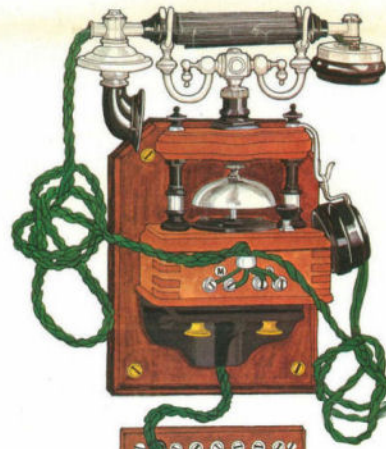
Handsets gave freedom of movement to telephone users, but early handsets needed individual batteries and were not successful when electricity was fed from the exchange. 1900.
