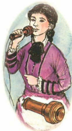
Bell's telephone was used as both a transmitter and a receiver. 1877.
