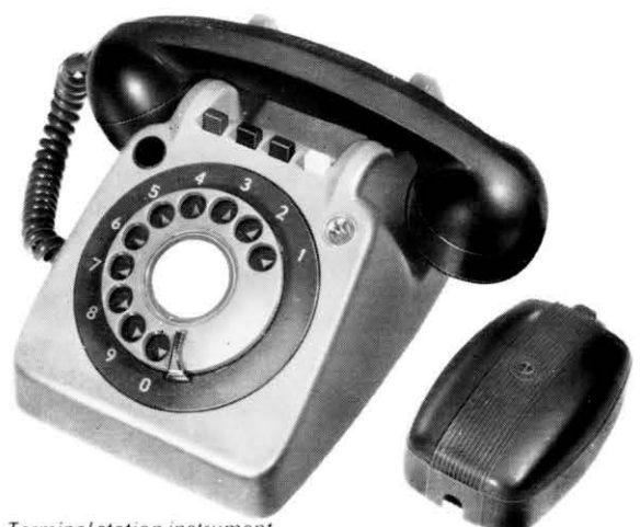
Terminal station instrument
