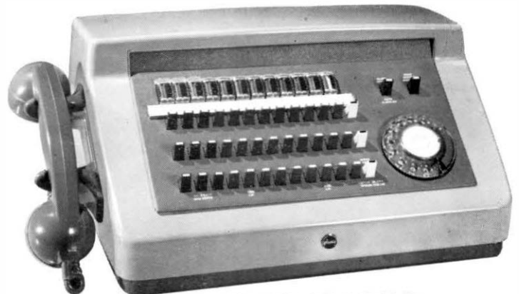
The 3+9 switchboard with five connecting circuits
