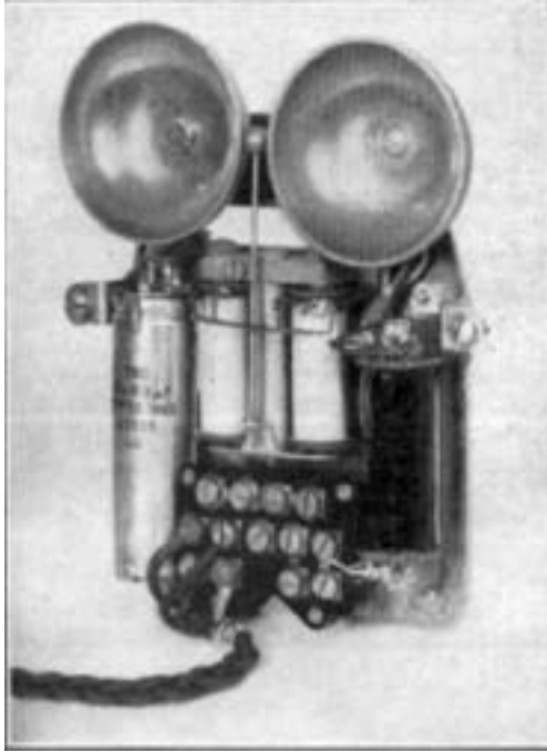
FIG. 20 - CHASSIS OF TELEPHONE NO. 700
