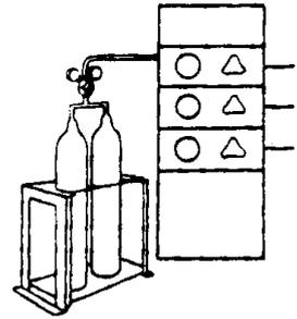
The high standard of maintenance essential to trunk cables and other high security cables means that it is appropriate to keep the sheath in near-perfect condition, and that the earliest possible warning of trouble is desirable. This is provided for by the use of alarm contactors at relatively frequent intervals along the cable route, so that the occurrence of a fault can be detected before the drop of pressure becomes widespread.
