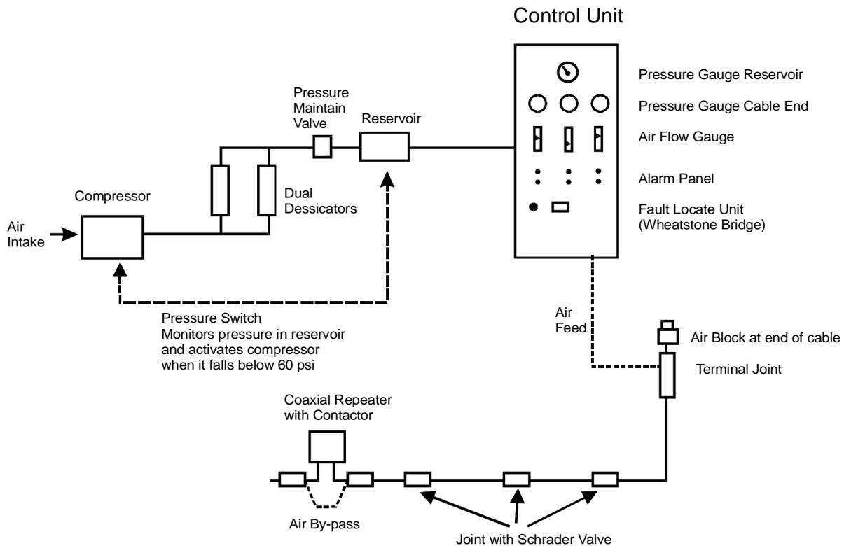
**Schematic Diagram of a Pneumatic Protection Network**
