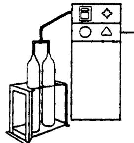
The scavenge system is a refinement of the static system. Whereas in a lead sheathed cable a static pressure is sufficient to provide protection until the development of a serious leak, in a plastic sheathed cable the moisture permeating through the sheath into the cable must be swept away continuously if a build-up of humidity is
