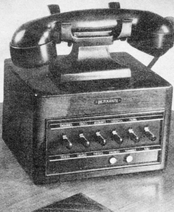
The Dictograph sub-station shown above is model HL 10/2, communicating with 10 other instruments. The full range of substations connect with between four and sixty-four stations. Other types are available to meet special intercommunication problems, details of which will be given on request.
