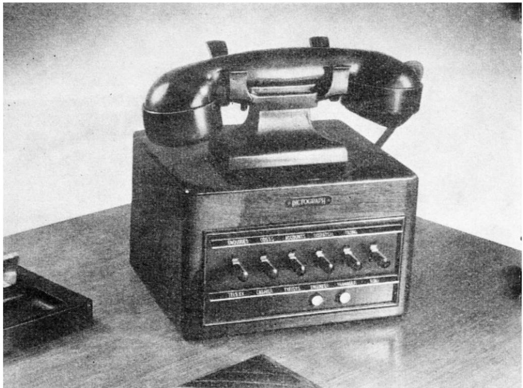
The Dictograph sub-station shown above is model HL 10/2, communicating with 10 other instruments. The full range of substations connect with between four and sixty-four stations. Other types are available to meet special intercommunication problems, details of which will be given on request.
