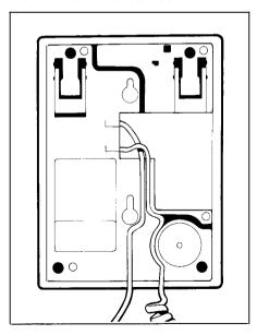
To prevent the handset from falling off the telephone when it is wall mounted, position the handset guide which is located above the words British Telecom by pulling it out and rotating it until it clicks. The diagram below shows how to do this. (The hook on the handset guide fits into the groove on the handset.)
