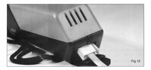
When the headset is plugged in the loudspeaker will continue to click at a low rate as a reminder that the amplifier is switched on. (Otherwise you might not be aware of this once you have removed the Receiver Headgear and the battery would discharge)
