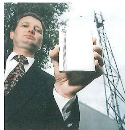
Figure 2—Passive picocell base unit with existing GSM base station in background
