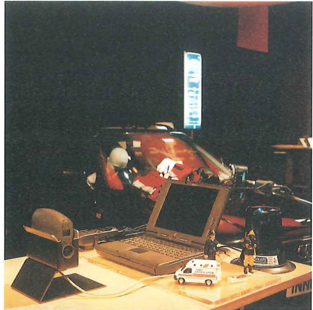
Traumalink, now in trials with Norwich and Norfolk Hospital, transmits high-quality digital pictures from the ambulance at the scene of an accident, directly to the consultant in accident and emergency, thus describing the whole scenario.
