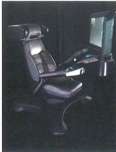
Figure 2—SmartSpace chair using transaural processing
