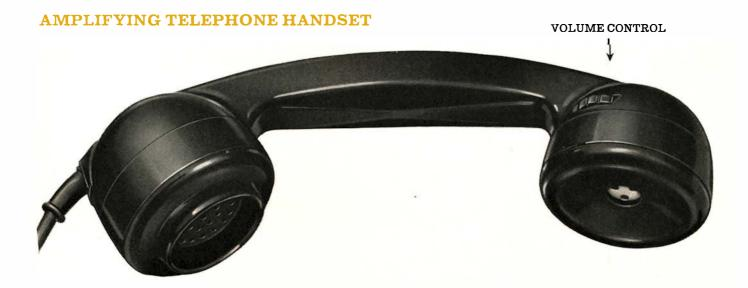
The amplifying handset helps customers who cannot hear very well and find difficulty in using a telephone. It is used with the modern telephone in place of the usual handset. The appearance is the same except for a small thumb-wheel volume control on the side of the earpiece. The sound in the earpiece is boosted by a transistorised amplifier inside the handset. The loudness can be regulated to suit the user
