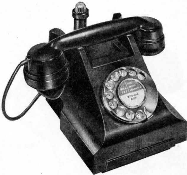
An ordinary telephone with low-voltage lamp attachment
