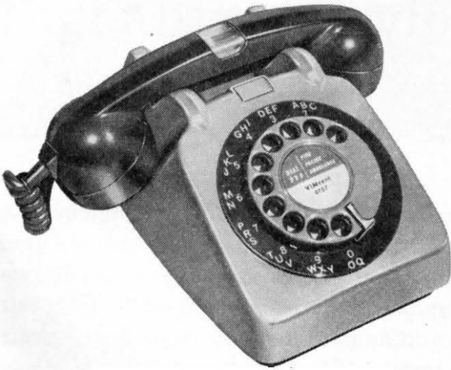
Modern telephone with neon lamp under transparent plastic cover in handset
