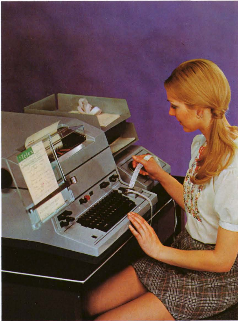
The photograph on the front page shows the modern basic telex installation with Teleprinter 15. The photograph above shows a Teleprinter 15 with integral reperforator and automatic message-transmission facilities. This equipment allows messages to be sent at a constant speed of about 70 words a minute—twice the speed of a good operator.
