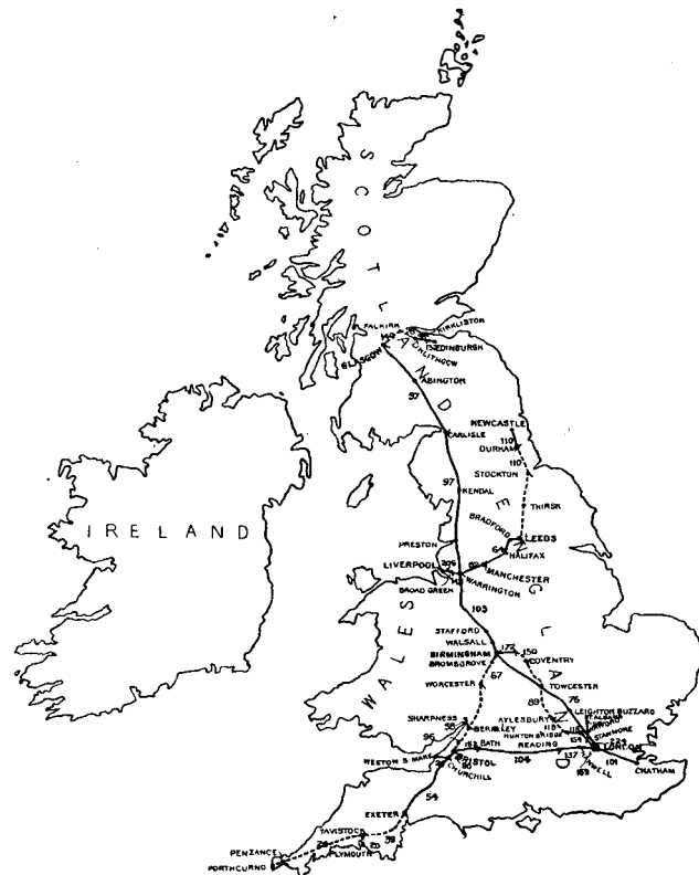
2.—1908. UNDERGROUND SYSTEM NOW EXISTING AND IN COURSE OF CONSTRUCTION. DOTTED LINES SHOW ROUTES IN COURSE OF CONSTRUCTION.
