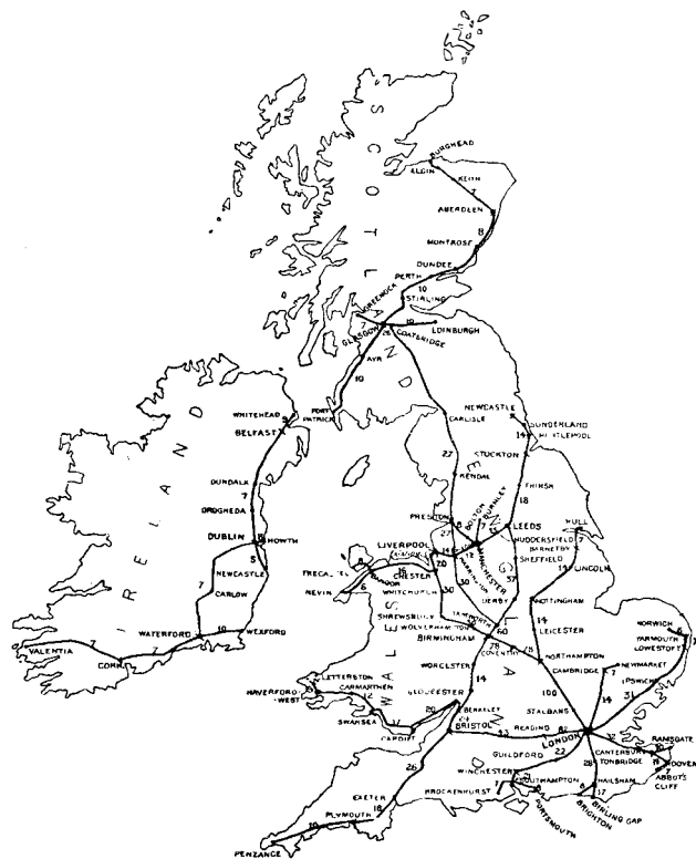
1.—THE COMPLETE PROJECT FOR AN UNDERGROUND TELEGRAPH CABLE SYSTEM IN THE BRITISH ISLES, PREPARED IN 1881. (THE FIGURES INDICATE THE NUMBER OF WIRES PROPOSED FOR EACH SECTION.)
