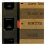
the progress of calls can he monitored using the loudspeaker – no need to lift the handset until the call is answered.
