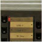
lamp signals to identify lines in use and the status of other terminals.
