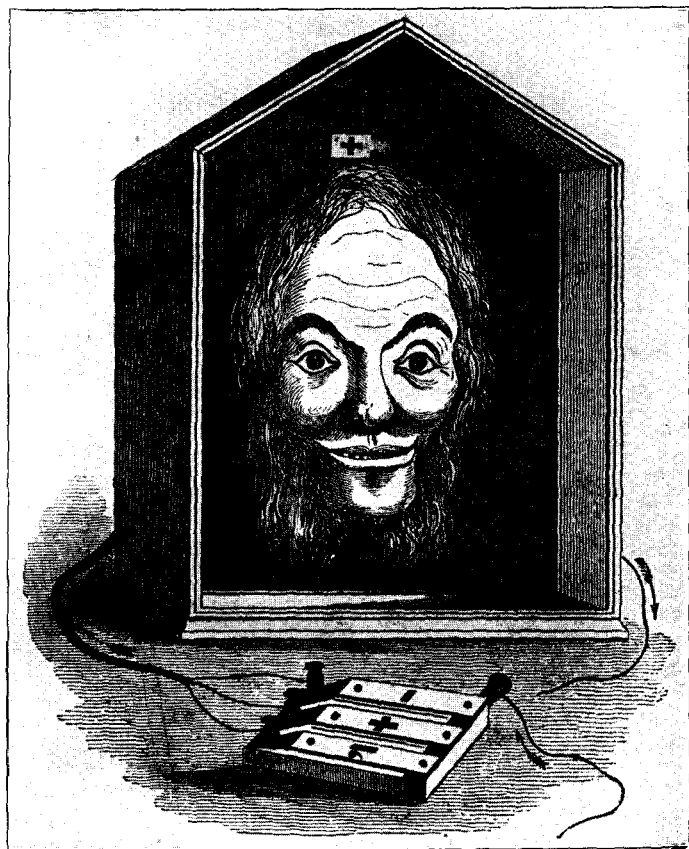
THE above illustration, a curiosity in telegraphy, is a reproduction from the Illustrated News of 1851 of the Comic Electric Telegraph by G. R. Smith. It was exhibited at the Great Exhibition of that year. Besides producing the actions of the eyes and mouth of the face, the instrument represented all the letters of the alphabet by means of combinations of the signs shown on the keys.
