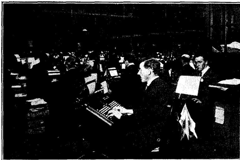
1.—THE LARGE TYPE OF MONOTYPE KEYBOARD MACHINES USED IN COMPOSING THE TYPE FOR THE TELEPHONE DIRECTORY. THE KEYBOARD IS SOMEWHAT SIMILAR TO A LARGE TYPEWRITER AND THE OPERATOR PUNCHES HOLES IN A ROLL OF PAPER ACCORDING TO THE LETTERS REQUIRED. THE PERFORATED ROLL IS AFTERWARDS TAKEN TO A CASTING MACHINE WHERE THE CORRESPONDING TYPE IS PRODUCED FROM MOLTEN METAL.
