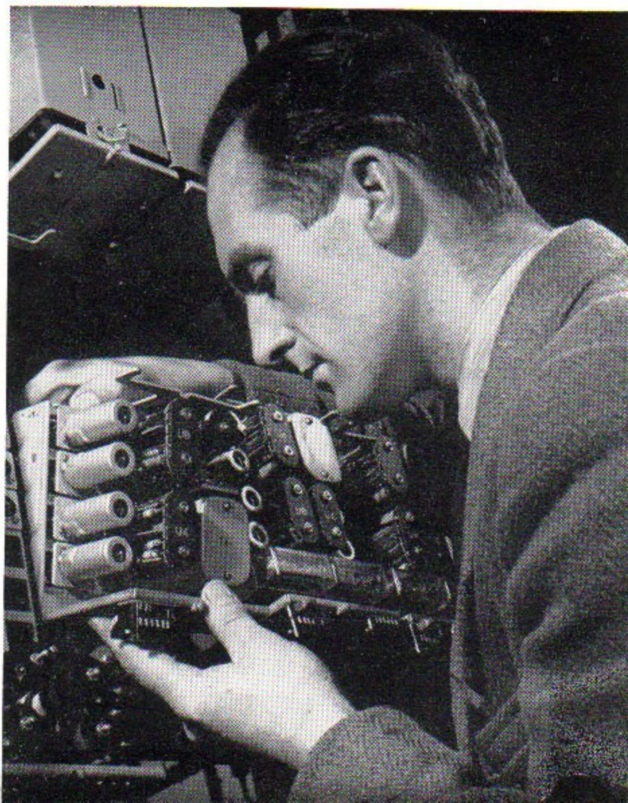
Expert and critical examination: an engineer inspects a single-frequency V.F. receiver before insertion into a test rack
