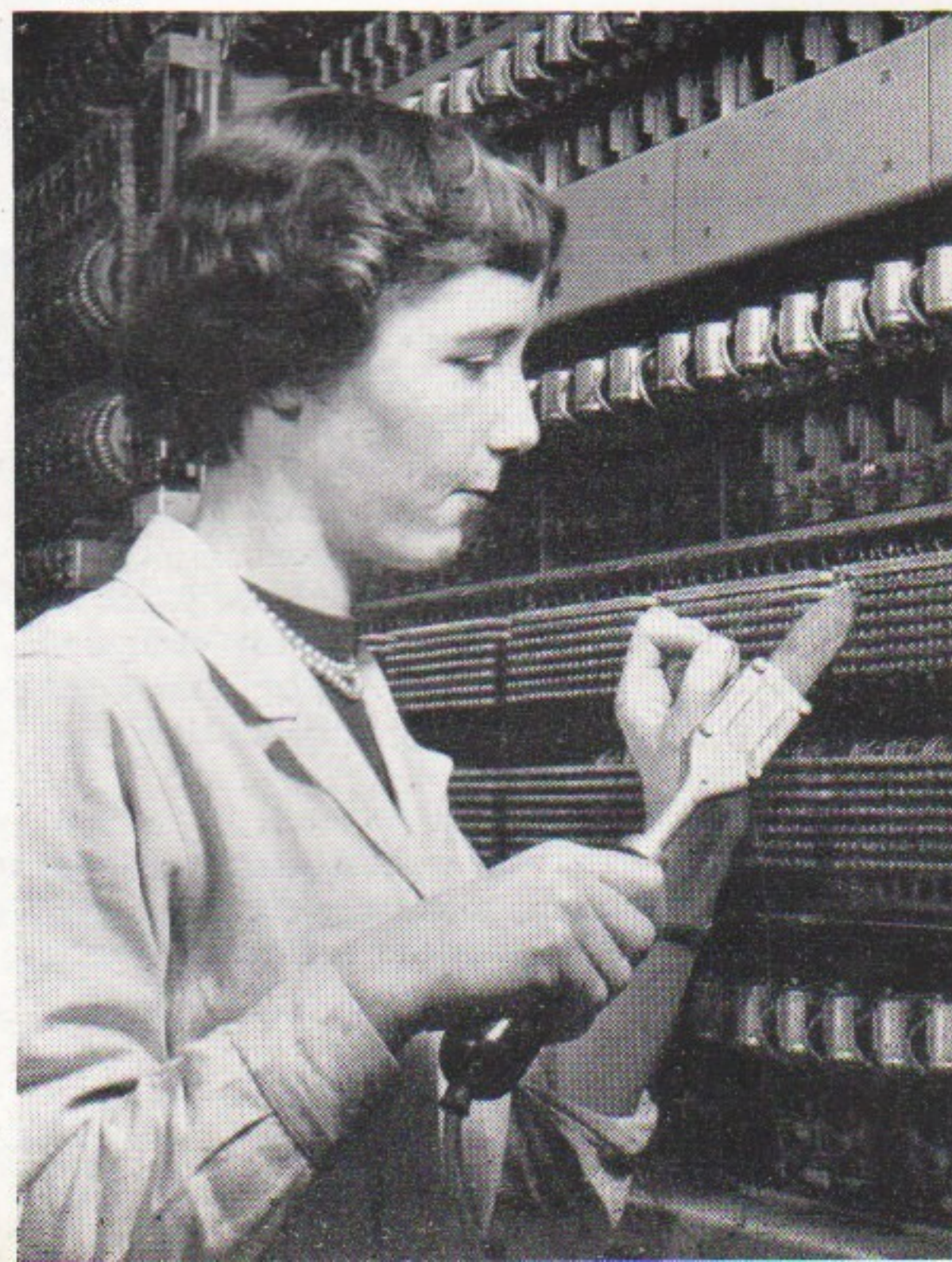
A good eye and judgment, combined with neatness, help this girl as she solders tag blocks on uniselector racks
