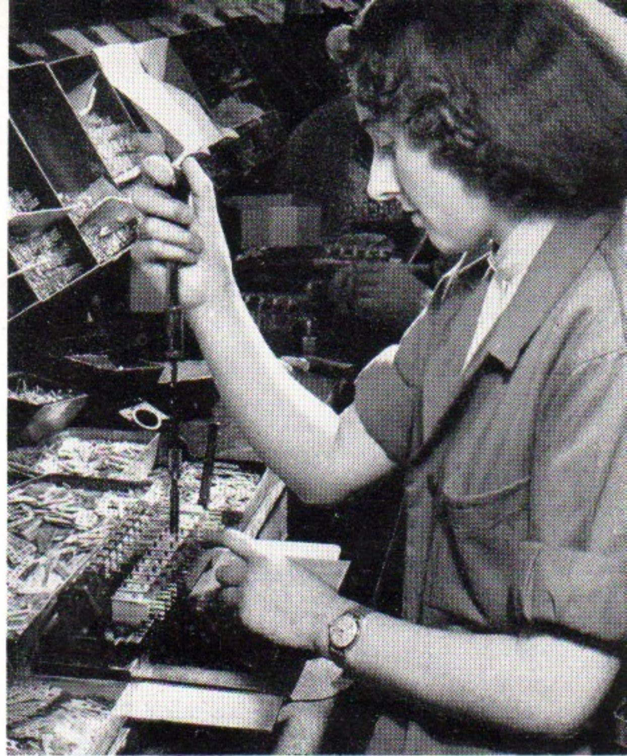
Nimbleness, speed and precision are the keynotes required when it comes to assembling these relay spring sets
