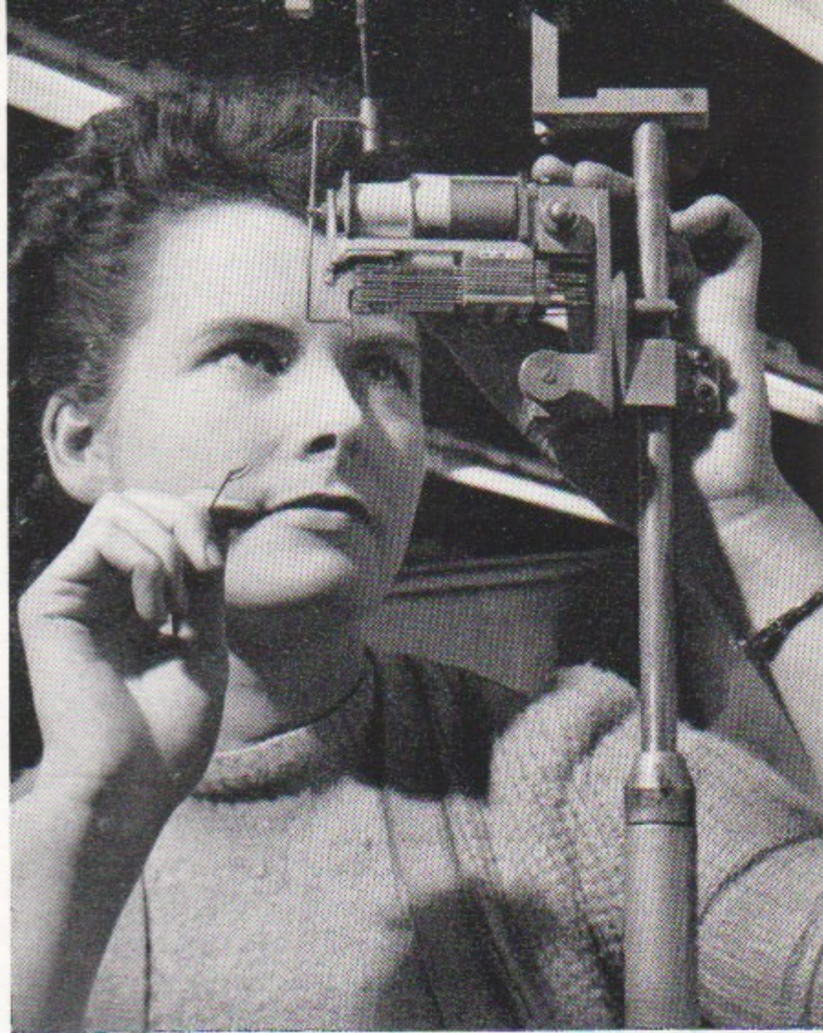
A study in confidence and concentration as this girl adjusts the contact springs of an automatic switching relay
