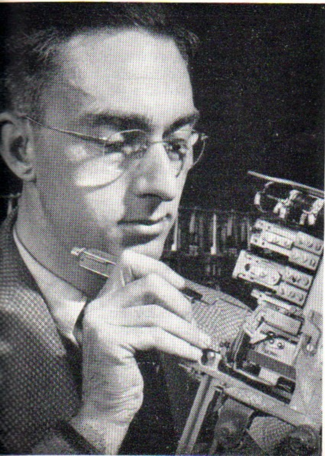
Delicacy of touch: an employee measures the spring tension of the rotary interrupter on 32A selector equipment
