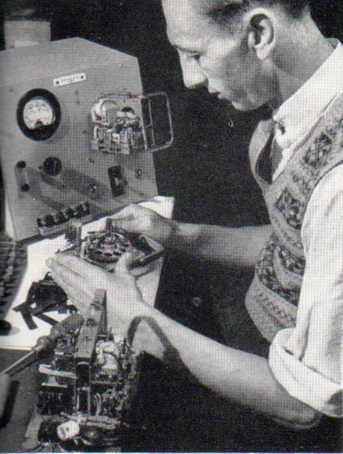
Intricate but intriguing: a skilled man engaged on mechanical adjustment and functioning test of the impulse regenerator
