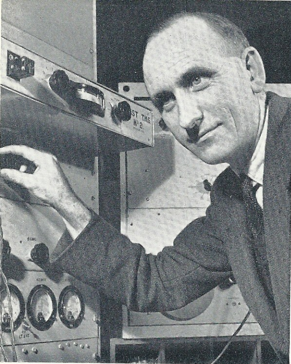
A member of Inspection Department (Transmission) listens for beats while testing carrier equipment.
