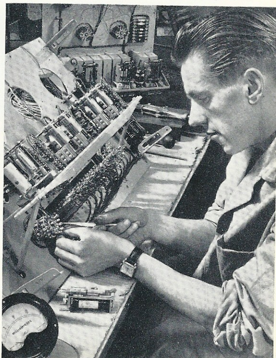
An employee at Pioneer Works, Wigan, wires a test set. Similar operations are done at Edge Lane
