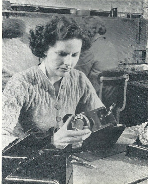
One of the telephone assembly processes. A girl from Department 26 places a dial in a telephone case
