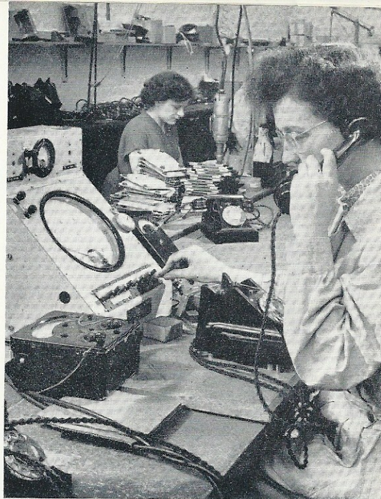
A telephone has been assembled and this employee carries out an important acoustic test
