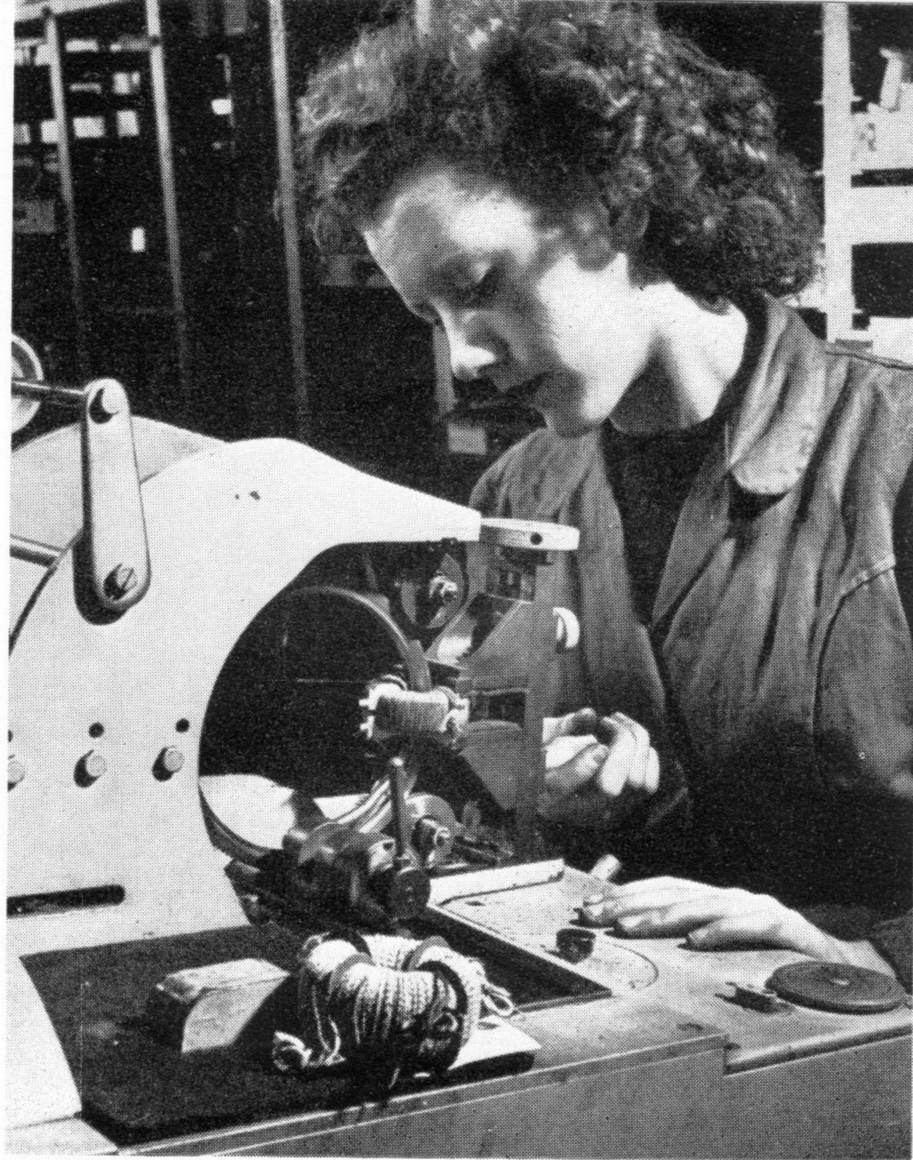
Winding toroidal coils for filters, using machines designed by A.T. & E.
