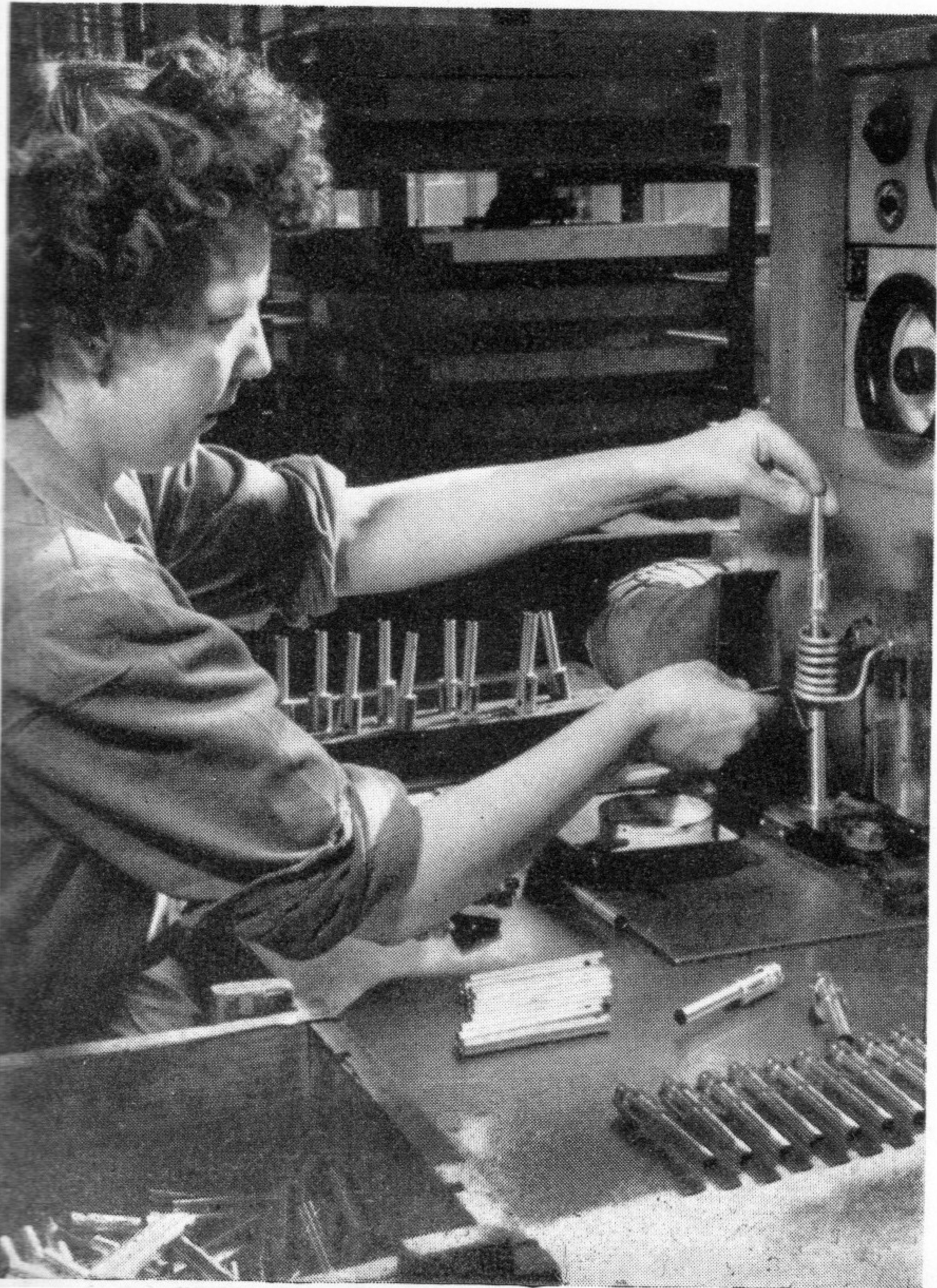
In Department 97: high-frequency soldering of rotary hub to wiper carriage
