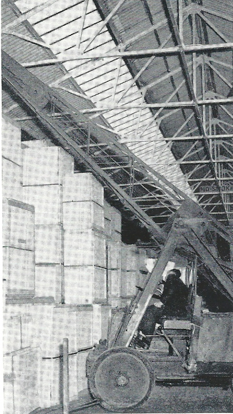
BIG HOIST Mobile cranes are used to reach some of the crates and save many hours each year
