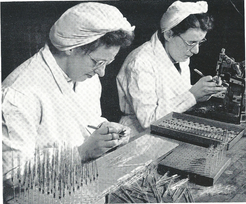
DEXTERITY AND PRECISION Two operators at Hivac engaged on assembling miniature valves. Steady fingers and eyes are needed for this task. Hivac's premises are among the best of their kind in Britain
