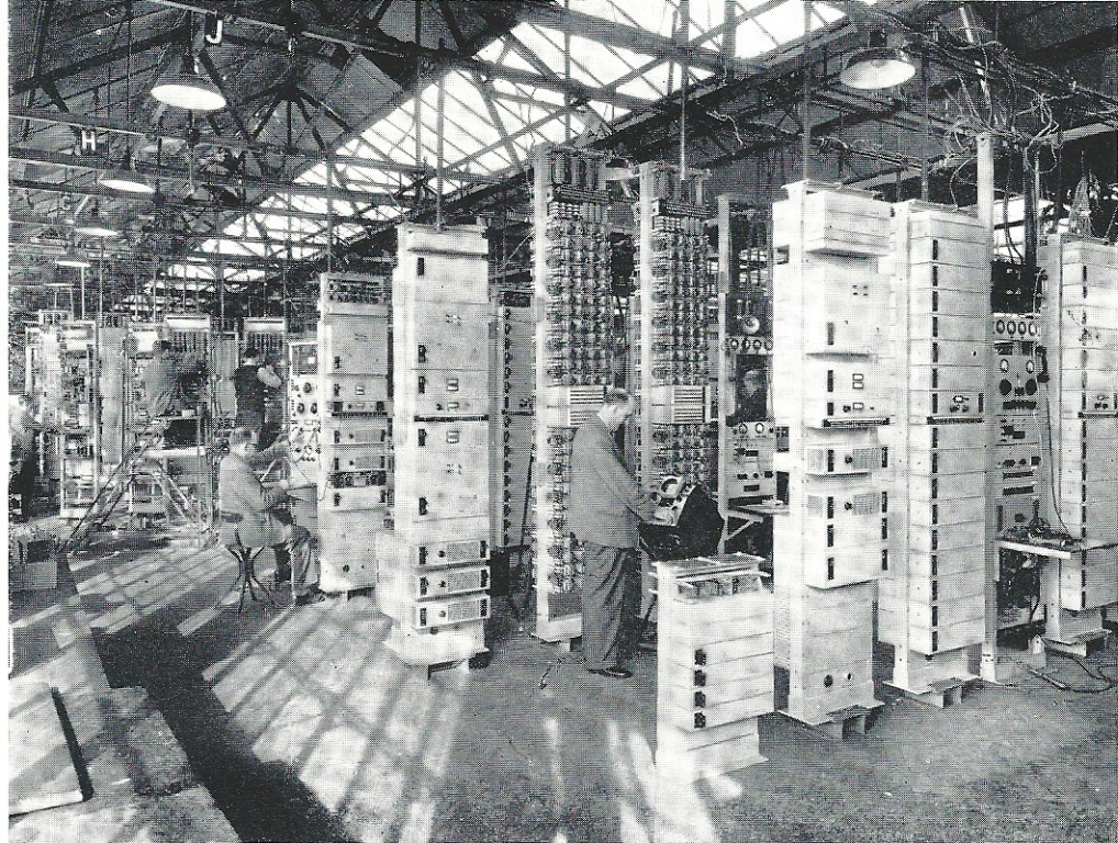
TRANSMISSION DIVISION The rapid growth of this division in post-war years has meant larger premises. Shown above is part of the Carrier Assembly and Wiring Department on the top floor at Strowger Works
