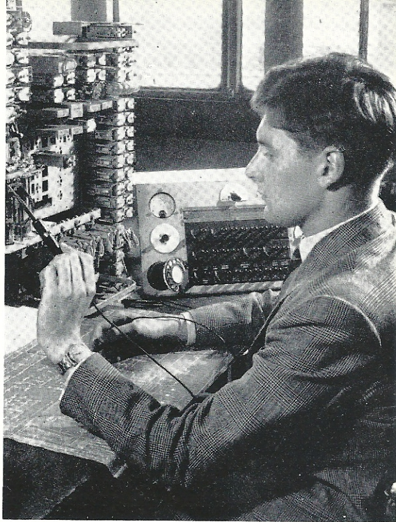
In Department 15, a final test is made on a Type 32A Selector
