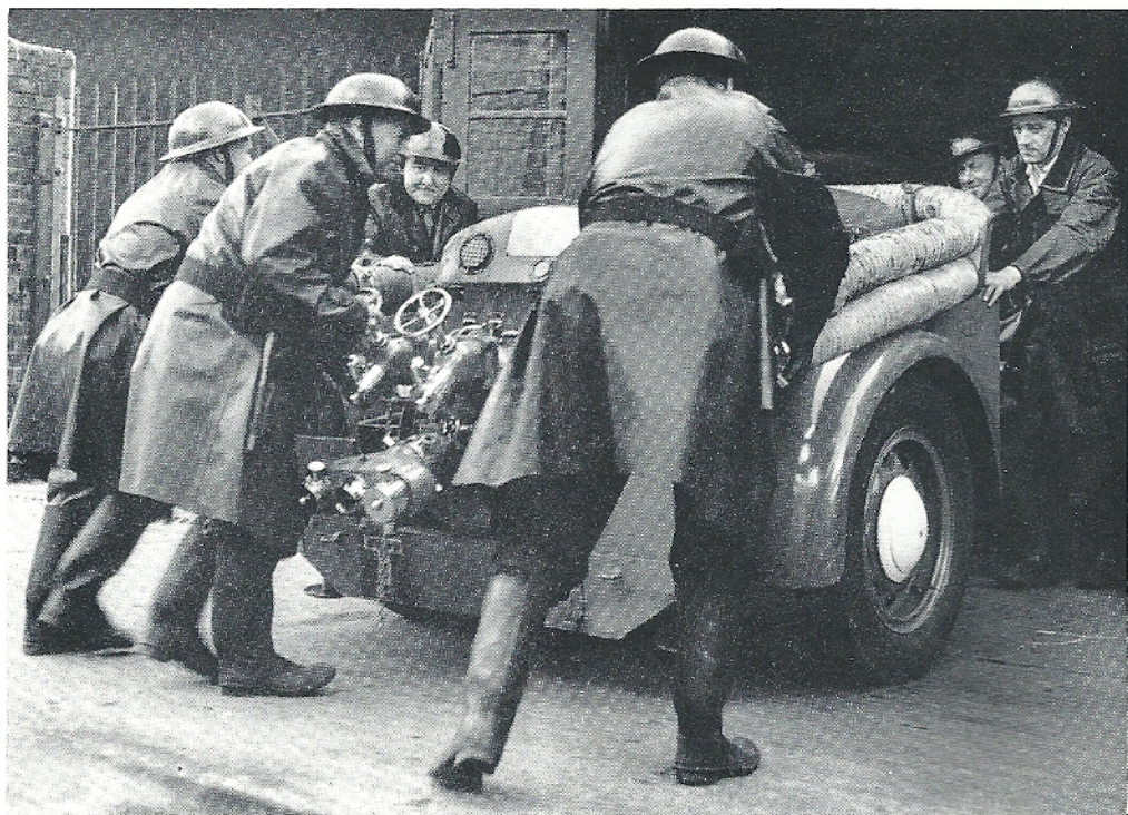
FIRE PUMP AND CREW A Harland fire pump, capable of turning out 400 gallons of water a minute, is brought out of the works fire station by a group of volunteer firemen, all specially trained for their jobs
