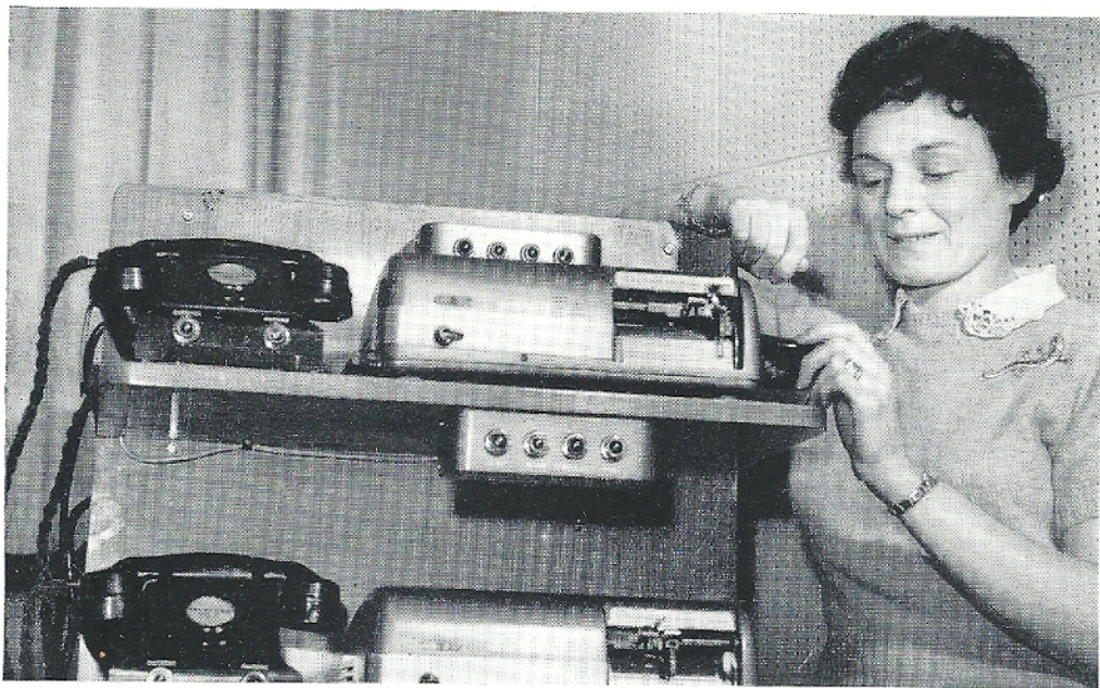
IN THE GROOVE Part of the experimental equipment which has been installed in Contracts Department at Strowger Works. Key personnel can now dictate letters on to specially-made records
