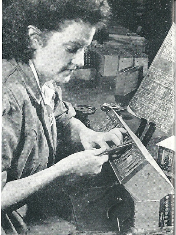
Wiring filters for line transmission equipment
