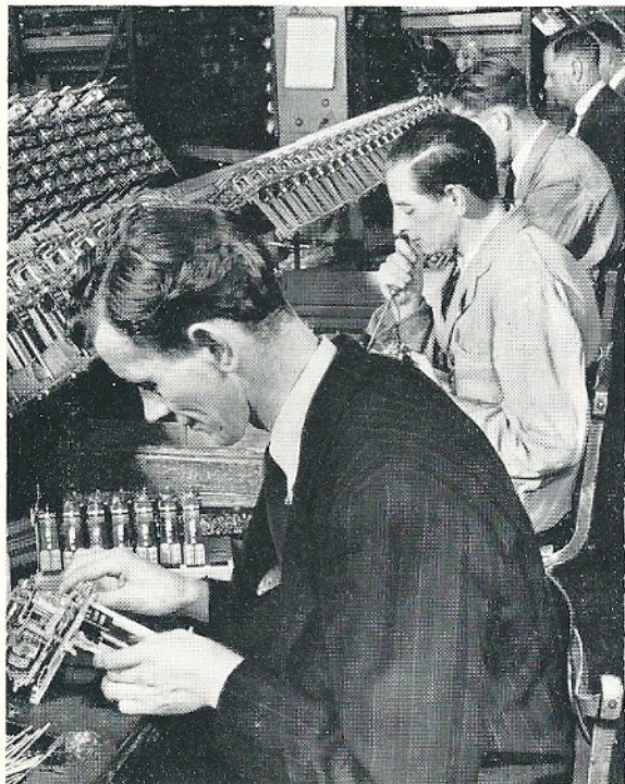
Type 32A Selector assembly and adjustment
