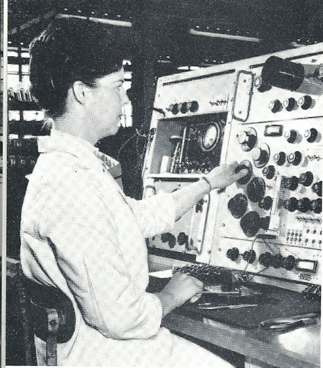
Mrs. Doreen Taylor testing transformers
