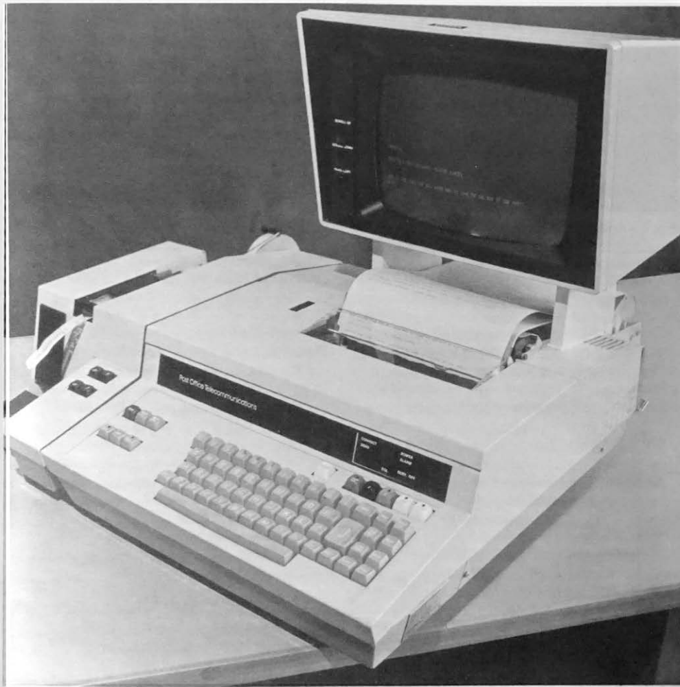
Fig. 1 – Teleprinter No. 31 with tape unit and VDU
