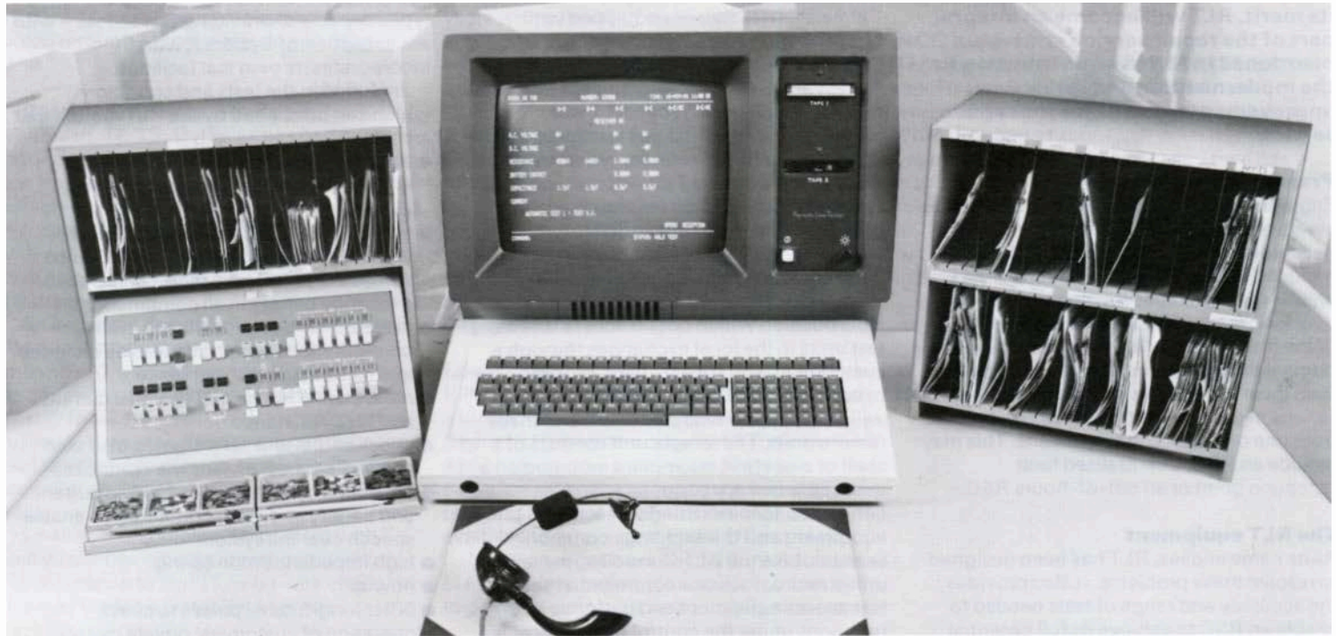
Figure 1. The desk layout used at Guildford – the Reception module is at the left and the RLT Controller in the centre. The pigeon holes are used for storage of fault cards and timesheets.
