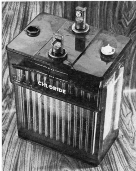
Figure 2. Split cell caused by arowths
