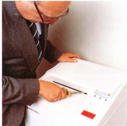
A shredding machine passes a test to ensure an operator's fingers will not be trapped.
