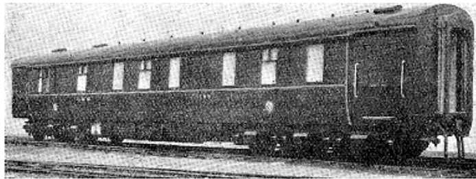
The Queen's saloon with protection plate shutters in open position.
