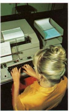
A private teleprinter system can provide continuous contact between two points. The customer has exclusive use of the circuit and pays no charge for the calls made. There is a connexion charge and an annual rental for each teleprinter. Charges for the circuit are based on distance.
