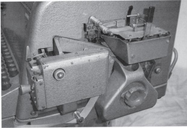
When the model 75 was required to operate with perforated paper tape, the appropriate attachments were factory fitted onto the right hand side of the machine, as shown in the picture above. The perforator was fitted towards the front, with the tape reader fitted towards the rear, and the "Chad box" for the punchings from the paper tape was fitted underneath the tape reader. The punches in the
